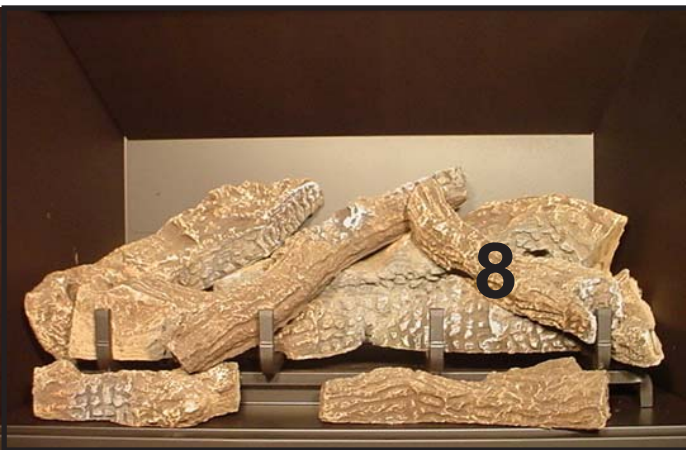
LOG #8 (SRV347-701): Hook log #8 on the right hand corner grate bar and rest its rear on log #1 as shown.
