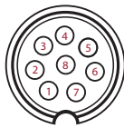
DP600 Binder Series 702 USB Connector 3 pin out information
