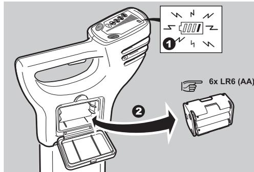
1. Replace or Recharge the batteries when the battery status indicator is empty.
