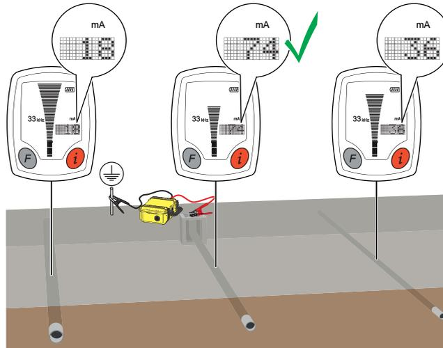
Additional information on the condition and layout of the service can be ascertained such as a fault in the service, damage to the insulation, or a connection off the service, these are typically indicated by sudden reduction in the current reading.
