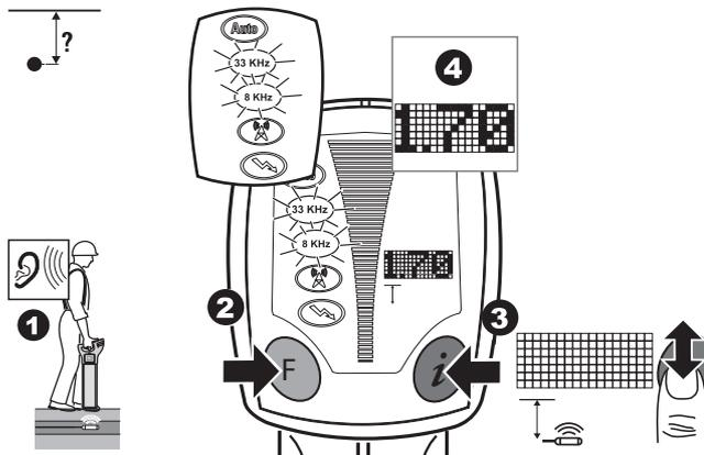
1. Switch on the sonde and set to the required frequency. Refer to "7 How to Use the Sonde" for more information.
