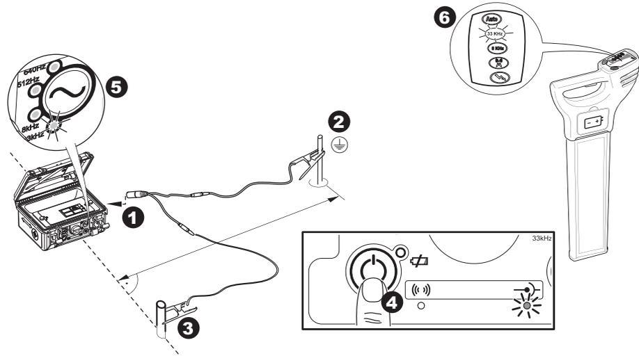
1. Plug the Transmitter's cable set into the connection socket.
