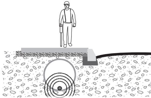
Take special care when the signal is produced by a sonde, lying in a large diameter conduit!
