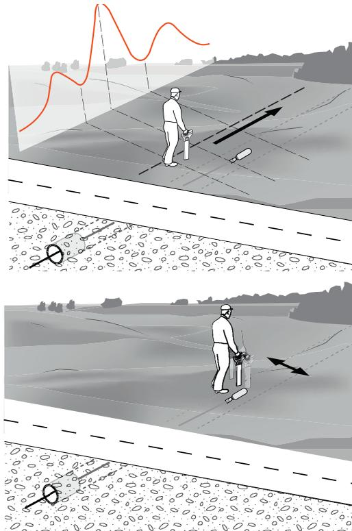
1. Walk in line with the suspected direction of travel observing the display. The signal strength indicator will rise and fall as you pass over the ghost signal at the back of the Sonde, the peak signal directly over the Sonde and the ghost signal at the front. The numeric signal strength indicator will display its highest value when detecting the peak signal.
