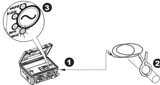
1. Connect the Signal Clamp to the Transmitter.
