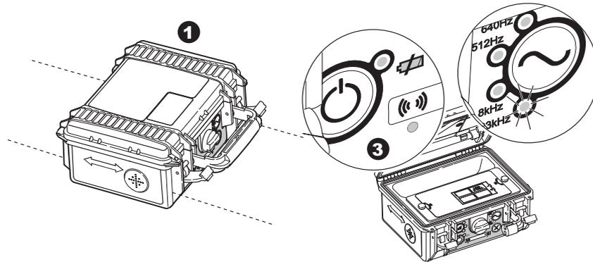
1. Switch the Transmitter on, observe the Induction mode LED is illuminated and the battery level is adequate. Change batteries when indicated.
