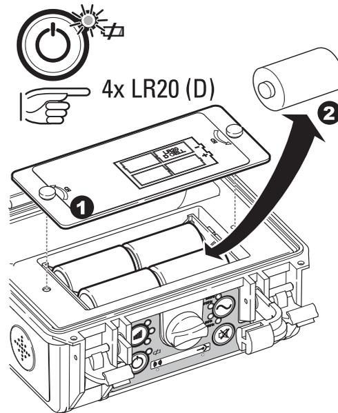
1. Unscrew the two fasteners and remove the cover.
