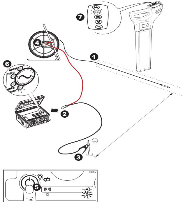
1. Insert the rod into the pipe, duct, conduit or drain until the desired length is in place.
