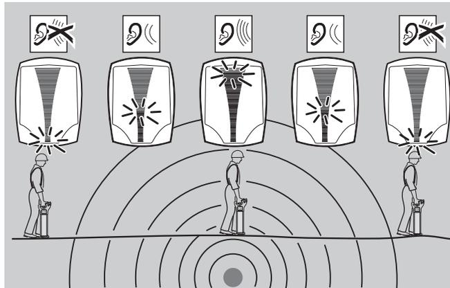
Retrace your steps to the area where the highest signal reading (peak response) was obtained. The service is directly below the Locator when the signal strength indicator is at its maximum. The audio output will automatically adjust to facilitate pinpointing over the service, and automatically reset when the signal strength indicator drops to its minimum position.
