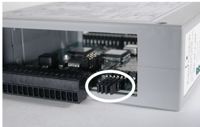
Figure 3.1 Jumper X2 Location (shown in Sourcing configuration)
