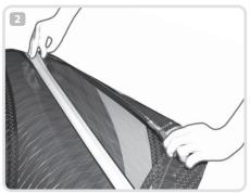
Next you **fold the head piece hard over** until the whole edge of the upper leech is smooth and tight. Use some force and after it gets bent a few times it will be easier. Hold the leech end of the batten to tension the edge against. While the edge is straight like this, start to roll it in.
