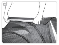
When you have a couple more turns and the roll is completely inside and supported by the batten pocket you can ease off with your left grip and roll the rest of the sail around itself.
