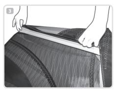
Now holding the head tight in your left hand, **roll the edge** in and continue to roll the sail around the top batten.
