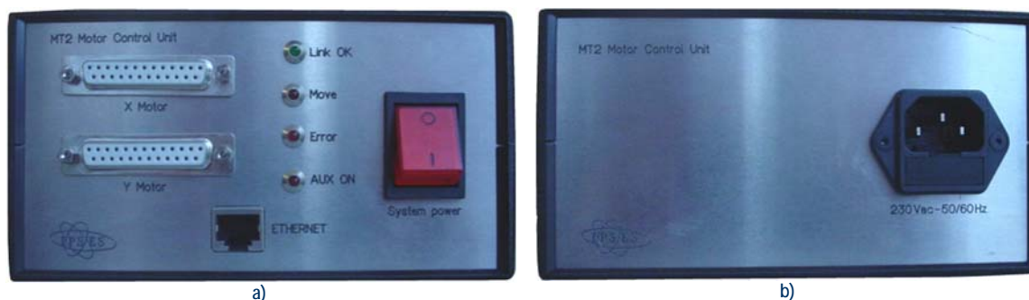
Picture 18: a) front and b) rear panel of MT2ETHMS box
