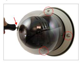
2. Carefully lift the cover. Using a screwdriver, remove the screw to detach the cover from the camera.
