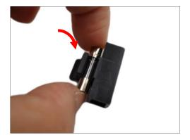
4. Insert the fuse holder back into the power adapter and push until it locks into place.
