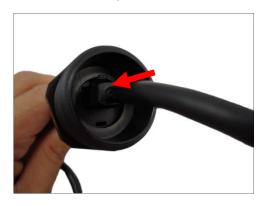
8. Insert the sealing rubber and claw into the cable gland body.
