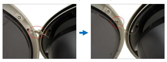
5. Tighten the four (4) screws to close the dome cover.
