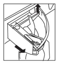
Swing open the detergent drawer and then remove the drawer by pulling it forward.
