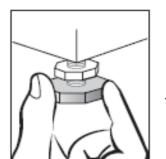
Adjust the feet to level off the washing machine.
