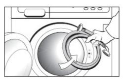
• The water inlet hoses will be inside the drum of your washing machine, when you receive the appliance.
