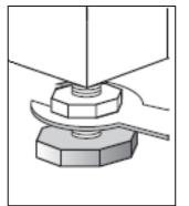
✓ Once levelled correctly, you should tighten the lock nut back up on each of the washing machine feet using a spanner.
