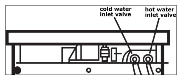
When you are facing the *rear* of the appliance, you will see two water inlet valves next to each other. The cold water inlet valve is on the left hand side and the hot water inlet valve is on the right hand side.
