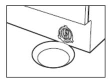
Place a container under the drain pump filter, to collect any excess water that may come out of the drain pump when it is removed.
