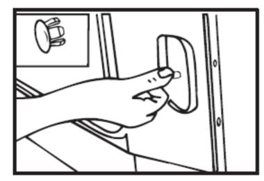
Insert the plastic caps that are supplied, into the holes that you have removed the transit bolts from.  $\checkmark\,$  Place the washing machine on a solid and level floor surface.
