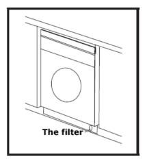
Locate the drain pump filter in the bottom right hand corner of the appliance.
