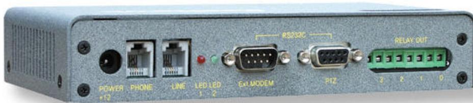
**Figure 1. VisionDial 3.x unit exterior**
