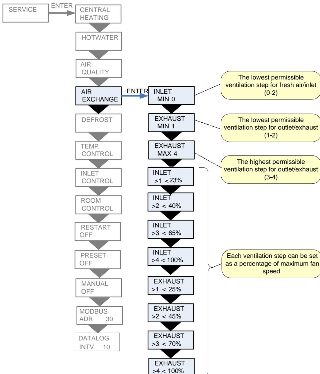
Figure 9: The "Air exchange" menu
