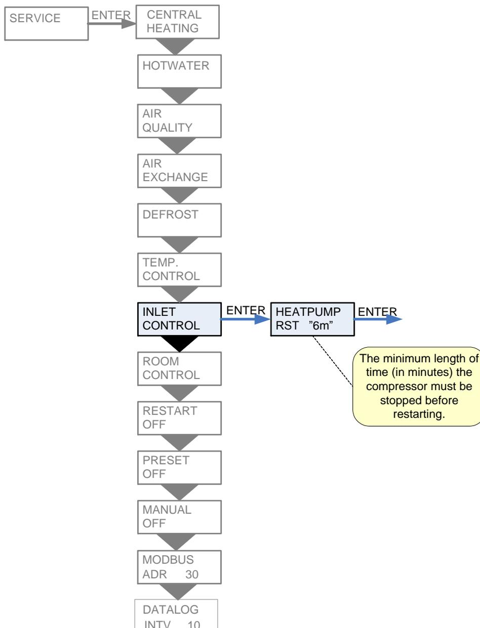
Figure 12: The "Inlet control" menu
