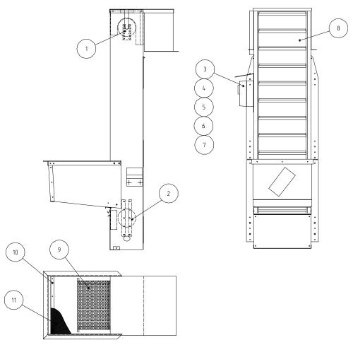
Figure 11: Elevator for machines with a flat top
