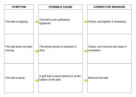
Figure 7: Fault analysis for Elevator.
