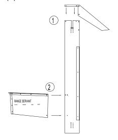
Figure 9: Mounting the ball duct
