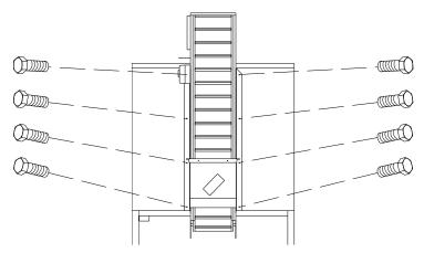
Figure 8: Fastening the elevator
