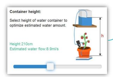
The water amount can be estimated in another way. Let the tube run past the device to the surface of the soil or to the base. Measure the watering time with a stop watch and then configure it in Daisy.si configurator.
