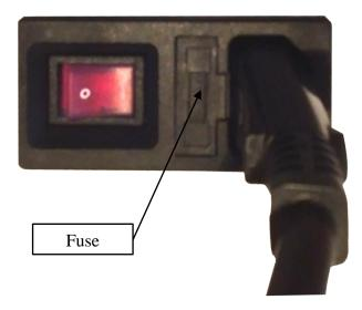
The power mains power connection is via an IEC connector fitted at the rear. Insert the supplied power lead and connect to a mains outlet. Switch on the supply at the mains outlet, and then operate the mains switch on the unit. The switch will illuminate if power is present, which means that the unit is in standby mode.
