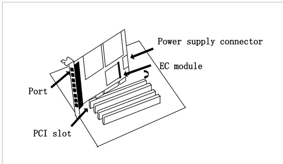
**Figure 4 Hardware setup**
