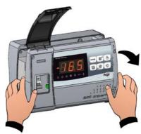
**Fig. 5:** Press on the sides of the hinges to remove them from their seats and so remove the front panel completely.
