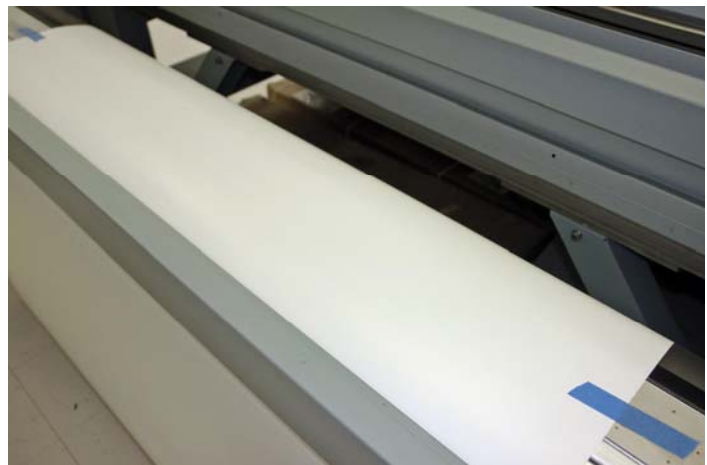
Figure 1 Tape the media edges
