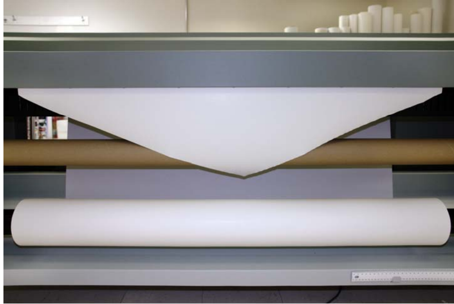
Figure 2 Cut the media at an angle
