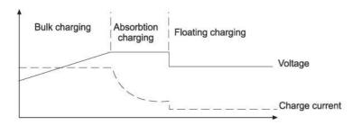
Bulk Charging Stage: charged the battery with current of 25A. When finished, the battery is 80% charged
