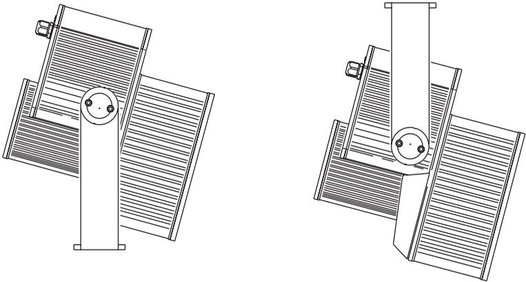
*When the fixture is located above the area to be illuminated, install with the power section on top.*
