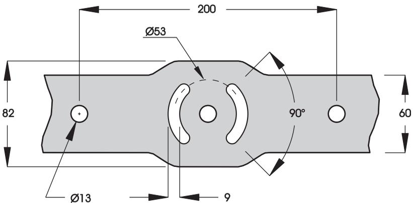
The Exterior 200 may be permanently fastened to any flat surface, pedestal, or other support that can safely bear at least 10 times the fixture's weight.
