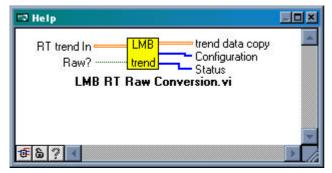
The "LMB RT Raw Conversion.vi" transforms data taken from LMB ADC node using Trend Tag.vi. If "Raw? Input is false data are converted to real to real voltage. On the output this Vi puts Trend data (raw or real voltage), array of configuration bytes and array of status bytes.
