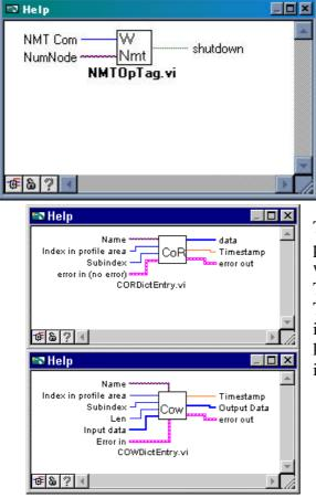
This Vi is to send a NMT message to a node or to all nodes in a bus.
