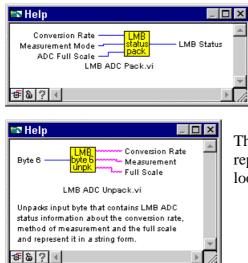
The "LMB ADC Pack.vi" is to pack the ADC setting in one byte to write in LMB.
