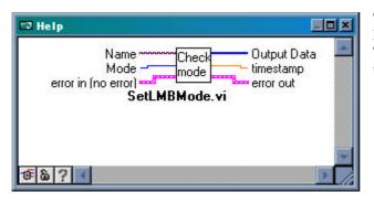
The" SetLMBMode.vi" is to switch a mode of LMB. LMB has sync and acync modes. This Vi saves the flash memory of LMB because in the beginning it checks the current mode.
