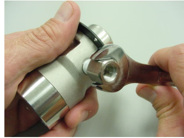
Remove the pump from the motor prior to tightening fittings
