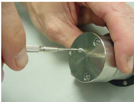
Internal pressure-relief valve: turn clockwise to close, counter-clockwise to open.
