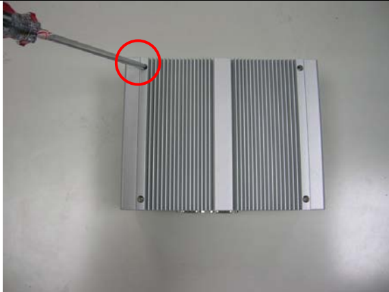
[Top] Unscrew four screws from the top.
