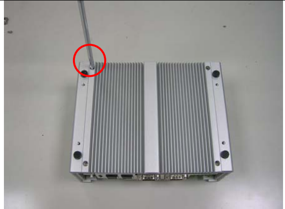
[Bottom] Unscrew four screws from the bottom.
