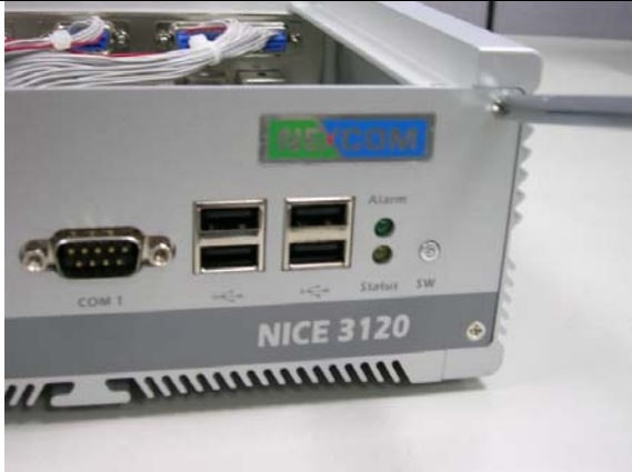
[Front] Remove four screws from the front panel.
