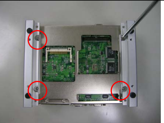
[Front] Remove four screws from the front panel.
