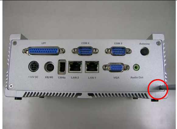
[Rear] Remove four screws from the rear panel.
