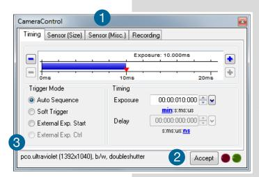
The camera control dialog always adapts to the camera type connected. For the pco.ultraviolet the camera control settings are spread over four *property sheets* 1, which will be explained below.
