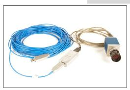
The *Adnaco-SU1* is a FOL Extender for USB 1.1./2.0/3.0 devices. It contains two components: the *Adnaco-UT1* (USB Converter) with power supply and the *Adnaco-UF1* (active USB 3.0 FOL cable (integrated electrical optical converter with length of 10, 30, 50 and 100m).
