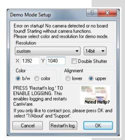
When CamWare is started, it automatically recognizes the camera type of the connected and running cameras.
