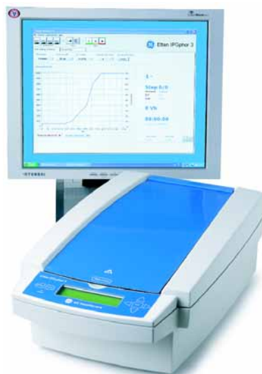
Fig 5-1. IPGphor 3 isoelectric focusing apparatus and IPGphor 3 Control software.
