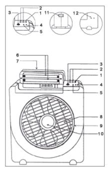
C. UPS / EXTERNAL POWER: 12 Volts DC Uninterrupted Power Supply is available across the terminals (12) for various applications as described in the introduction. In case the EFL's own battery is discharged, the product can still be used on external 12 Volts supply.
