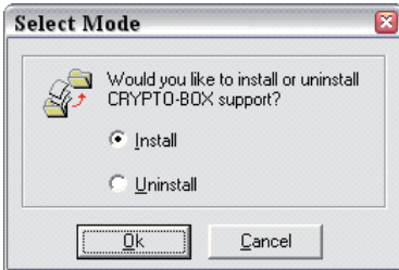
Fig. 2.1 Installing the dongle drivers manually. CbSetup.exe - Select Mode - Click "OK" to confirm
