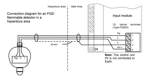
The use of barriers to create an I.S. supply imposes certain restrictions on the parameters of the interconnecting cables used. Consult the barrier manufacturer's data for further information.
