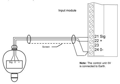
For systems operating at 24V, the maximum cable loop resistance is therefore (24-8)/25mA i.e.  $640\Omega$ .
