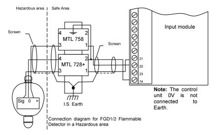
In order to maintain intrinsic safety, the capacitance and inductance or inductance to resistance (L/R) ratio of the loads connected to the terminals of the FGDIO barrier must not exceed specified values:
