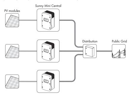
The Sunny Mini Central may only be operated with PV arrays (modules and cabling) of protection class II. Do not connect any sources of energy other than PV modules to the Sunny Mini Central.
