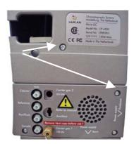
2. Mount the bracket with the two screws (M4x12mm).
