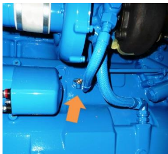
Fig. 13 Draining of coolant from the engine block and filling mixture intercooler
