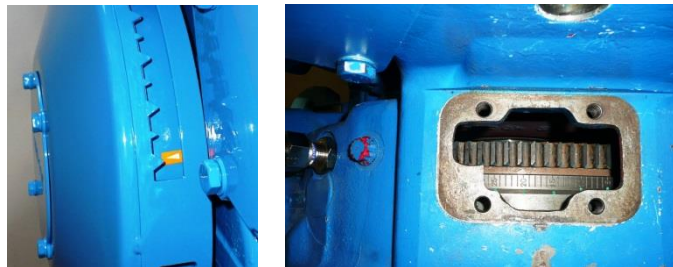
Fig. 8 Setting the advance using the scale on a crankshaft torsional vibration damper or on a flywheel
