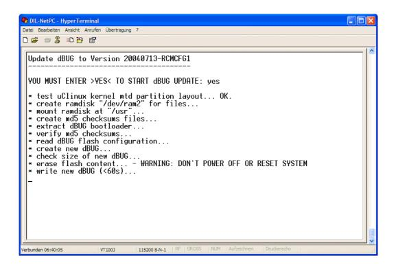
• **8.** Step: After the dBUG ROM Monitor in-application programming process has finished, it is necessary to reset your IGW/800 or IGW/900 Linux Device Server to run the new flash software.
