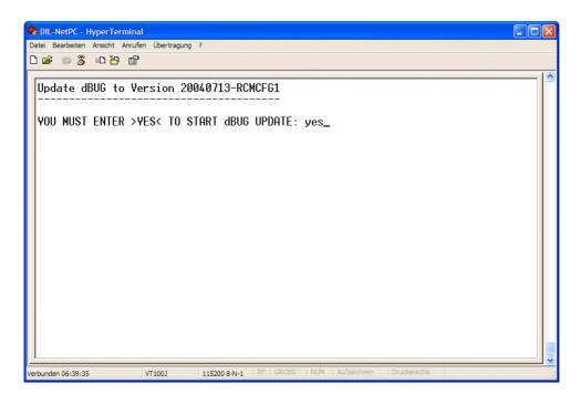
• **7. Step**: Please wait until the dBUG ROM Monitor in-application programming process finish's without errors.
