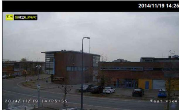
Camera view with three overlays: Image overlay (top left), Date & time (bottom left), and Text string (bottom right)
