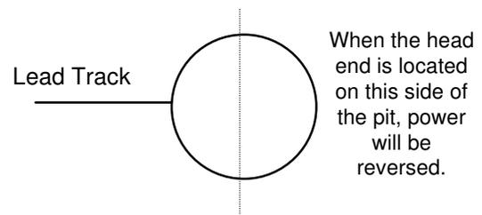
**Optional Mode:** In this mode, sometimes called “toggle” mode, the ATR operates by remembering where you start each move, and *toggles* the power if you move more than 90 degrees in either direction from the starting point of that particular move. For example, if you were to turn a locomotive 180 degrees from any track location, the controller
