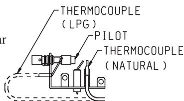
7. Depress and turn gas control knob counterclockwise to "PILOT". A spark is produced when gas control knob is turned between "IGN" and "PILOT". Repeatedly depress and turn gas control knob between "IGN" and "PILOT" until pilot is ignited. Continue to hold the control knob in for about one (1) minute after pilot is lit. Release knob and it will pop back up. Pilot should remain lit. If it goes out, repeat steps 2 through 7.
