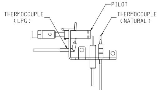
8. Hold the control knob in for an additional 10 seconds to prevent the ODS pilot from shutting off the gas while the thermocouple is warming up.
