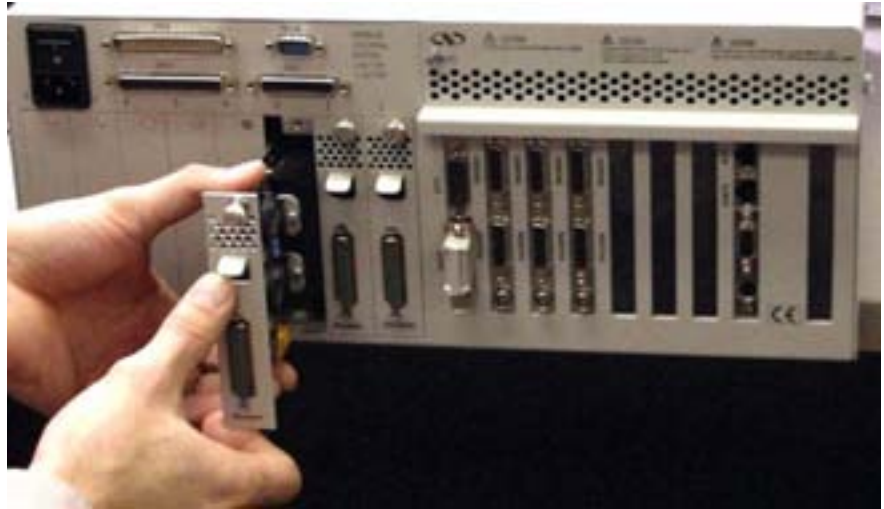
Figure 11: Installing Driver cards.
