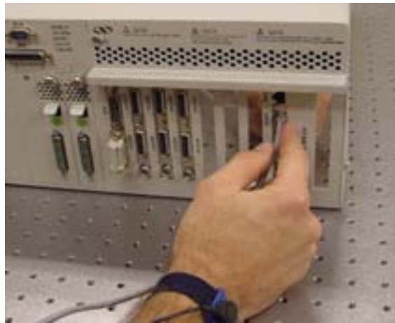
Figure 15: Direct Connection to the XPS using cross-over cable and REMOTE connector.
