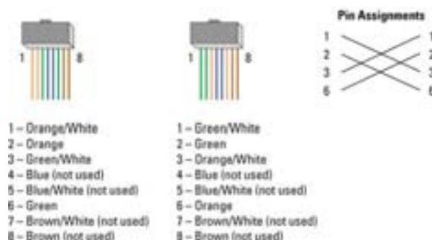
Figure 13: Ethernet Cross Over Cables.
