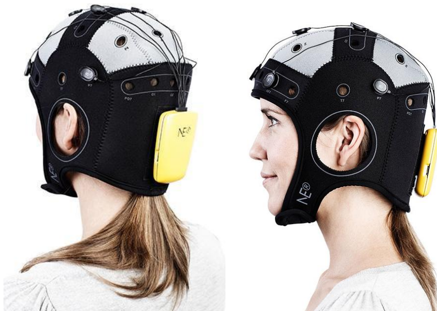
Figure 1. The Enobio wireless EEG monitoring system (Lt: posterior view, Rt: lateral view).
