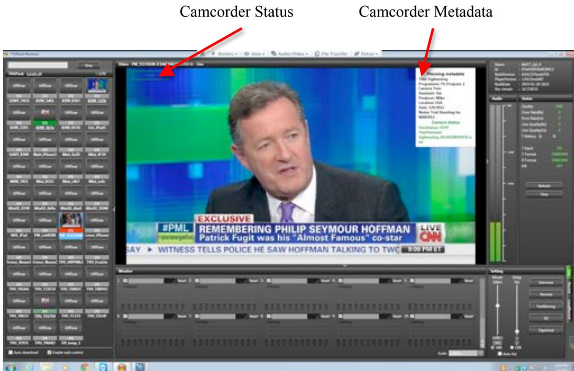
5. When live, if you mouse over the Preview screen, you should see more details about the camcorder connected to the TVU Pack including: Planning metadata, camera recorder status, cameras model type and more
