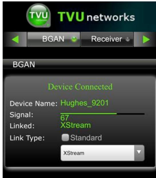
Note: If the interface connected with the BGAN device is consistently yellow and does not change to green after setting up the “Link Type”, please check whether the BGAN equipment - when connected to a PC - can work normally with LaunchPad’s X-stream mode.
