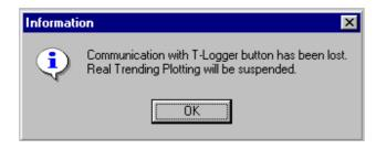
T-Logger Button must be always on Dot Receptor. If User place a T-Logger Button in other place during Real Trending, a communication error will appear and Real Trending graph will be finish.
