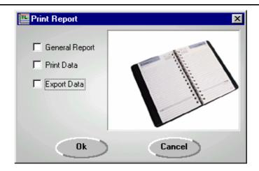
For a mission with 2048 data will be printed at 330 data points by page until completing a maximum of seven pages. **Export Data:** Allows the user to export mission data to a file disk. It will have the extension (\*. xls) compatible with Microsoft Excel<sup>TM</sup>. This file will be recorded on application directory/Reports.
