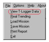
Allows user to set a Mission, read the information on the Mission, plot data or plot a histogram graph. T-Logger button must be inserted on dot receptor to obtain correct results. If the T-Logger is not on the dot receptor a warning message "Please insert T-Logger on Dot Receptor" will be displayed.
