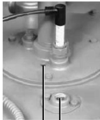
Burner Viewing Port Blast Tube Viewing Port
