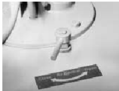
Secondary Air Adjustment for 4-30HP
