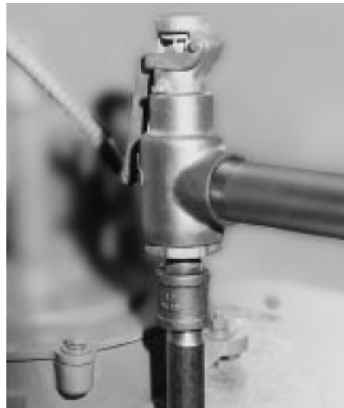
2) Remove the safety valve
