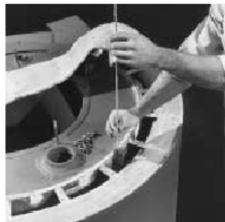
3) Remove clean out plugs and clean the bottom of combustion chamber.
