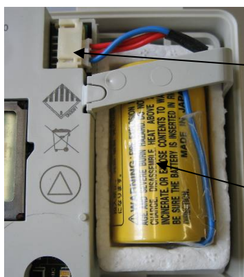
Picture 1: inside view with battery, calculator housing 2
