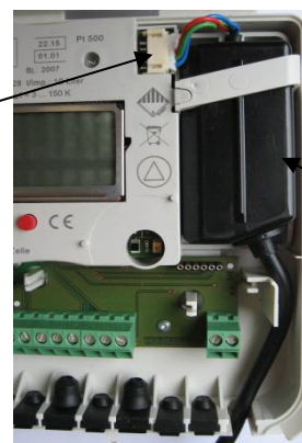
Picture 2: inside view with power module, calculator housing 2
