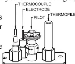
9. Push in control knob all the way and hold in. Repeatedly push the piezo ignitor button until the pilot is lit. Continue to hold the control knob in the for about one (1) minute after the pilot is lit. Release knob, and it will pop back up. Pilot should remain lit. If it goes out, repeat steps 5 through 9.
