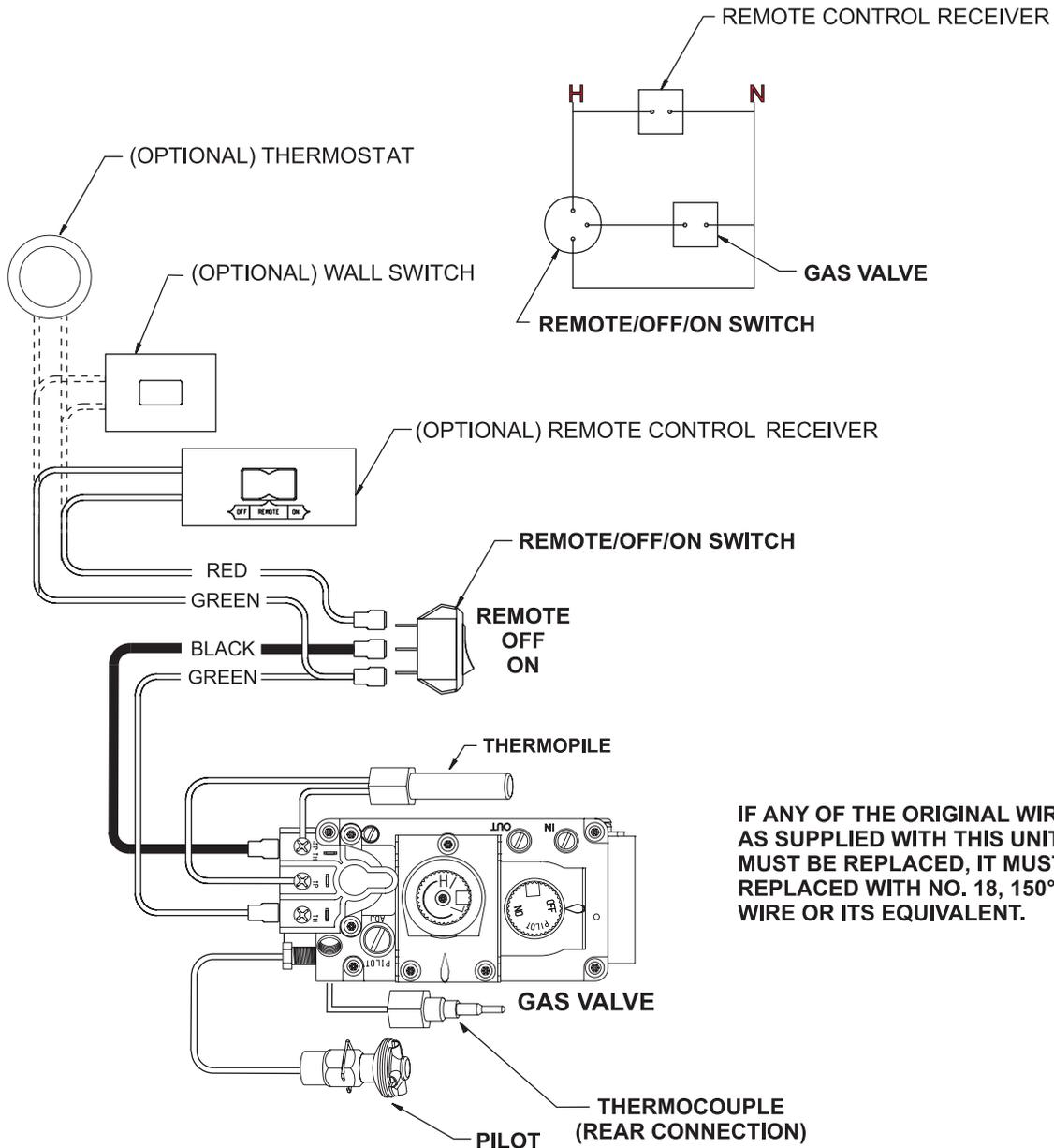
**IF ANY OF THE ORIGINAL WIRE AS SUPPLIED WITH THIS UNIT MUST BE REPLACED, IT MUST BE REPLACED WITH NO. 18, 150°C WIRE OR ITS EQUIVALENT.**
