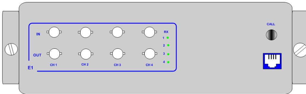
**Figure 10 - Data Interface Unit 4 E1 BNC + EOW**
