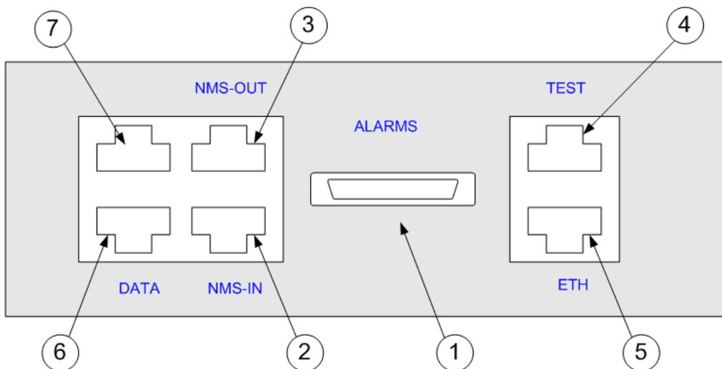
**Figure 4 - IDU Interface Connections**
