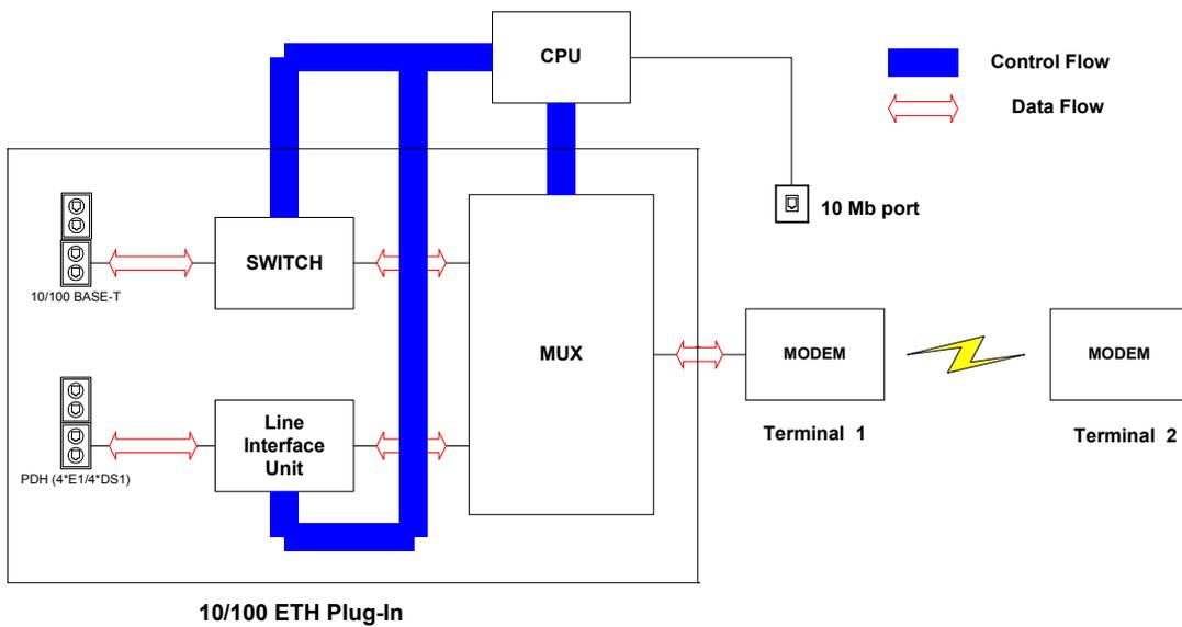
The Ethernet ports of the Data Interface Units are based on the Marvell Link Street 88E6063 7-port switch.
