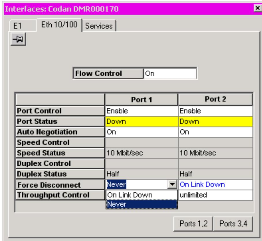
**Figure 77 - Ethernet Interfaces Port Configuration**
