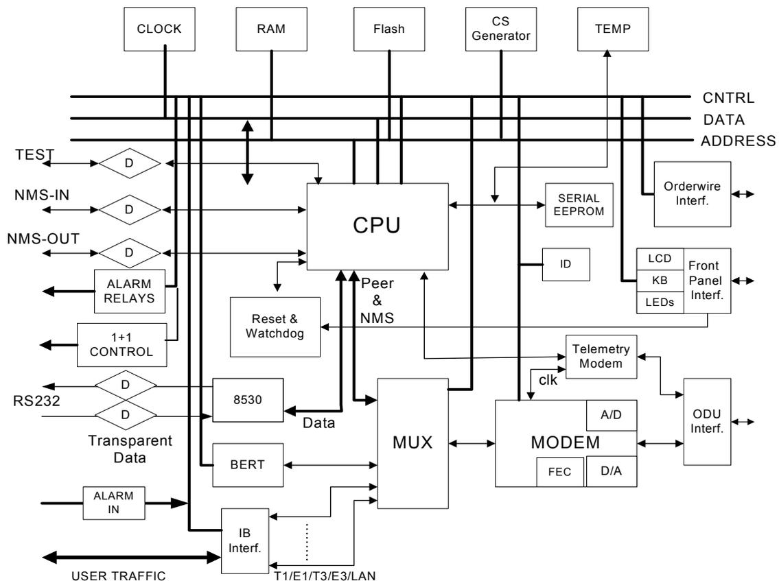
**Figure 8 - Digital Portion Block Diagram.**
