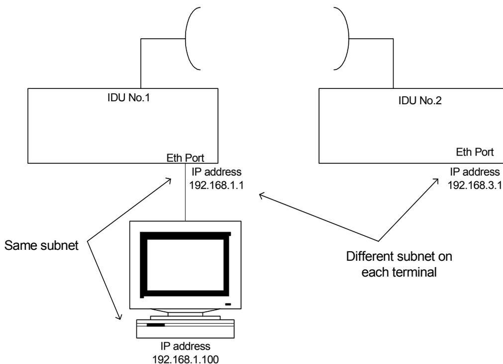
**Figure 62 - Out of Band Management via the Eth Port**
