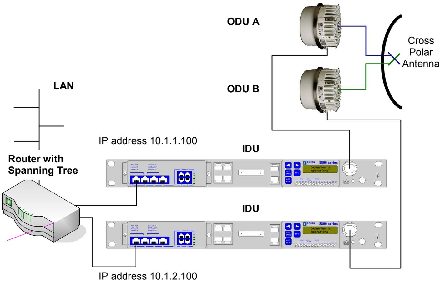
Figure 75 - Left Hand Terminal IP addressing example
