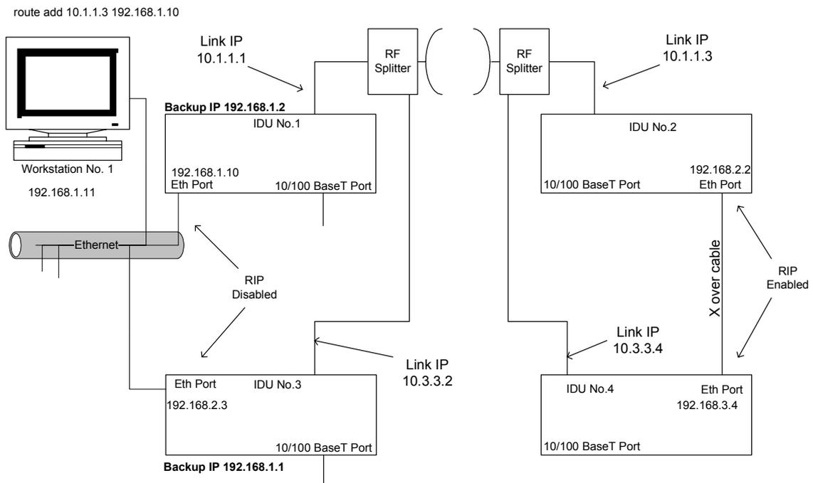
**Figure 65 - IP Configuration for protected system**
