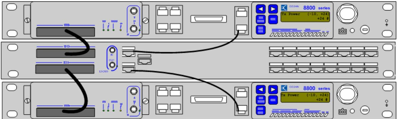
**Figure 69 - 16E1/E3, 1 + 1 with RJ45 Breakout Panel and Management Redundancy**
