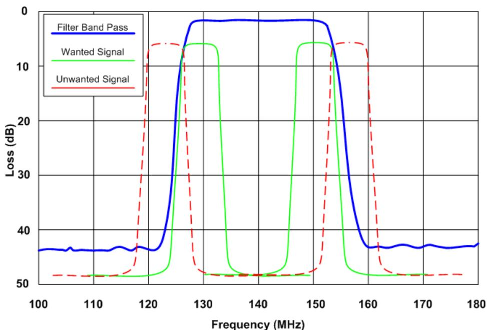
**Figure 33 - Adaptive IF Filtering Adjacent Channel**
