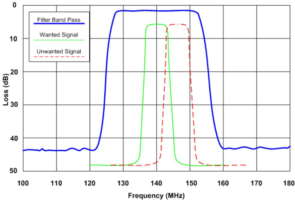
**Figure 32 - Required Signal plus Adjacent Channel**
