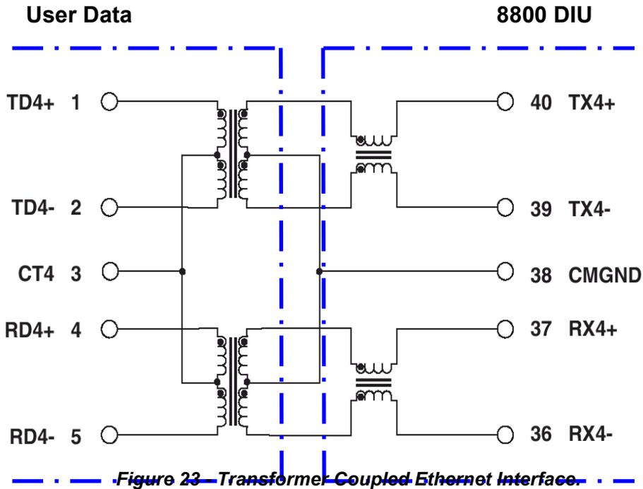
The following is the basic block diagram of the Ethernet Data Unit Interface:
