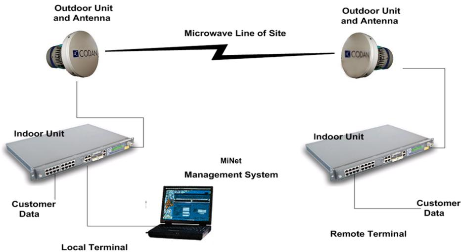
**Figure 1- Typical Codan 8800 series radio link**
