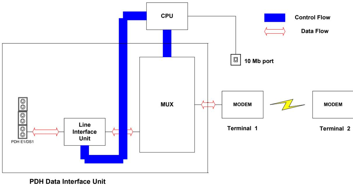
**Figure 19 - PDH Interface Block Diagram**
