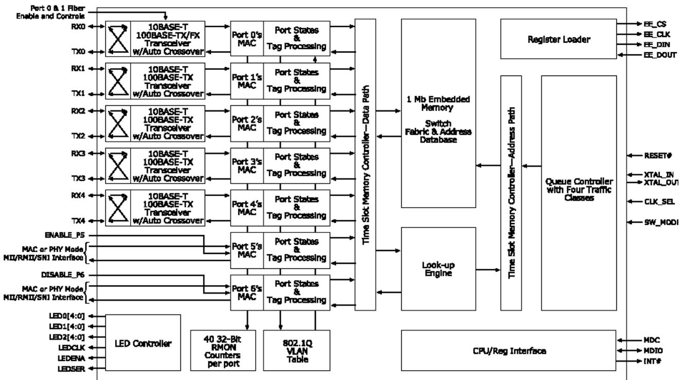
Figure 25 - Block Diagram of the Link Street 88E6063 7-port Ethernet Switch.
