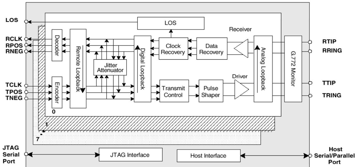
**Figure 20 - Block Diagram of the Cirrus Logic CS61884-4 8E1/DS1 framer.**
