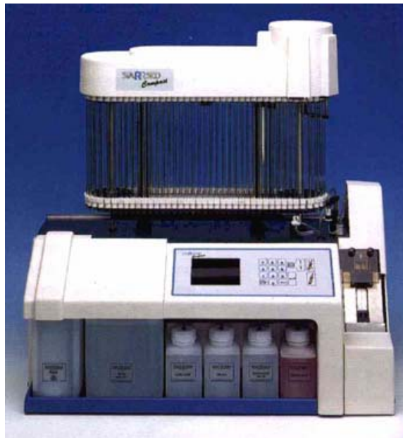
Figure 1: StaRRsed Compact ESR analyser
