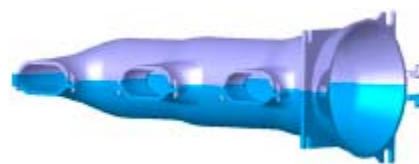
Fig. 16 Steam exhaust system for three mixing systems
