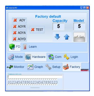
**Buttons to setting the type of communication** (AOY, AOYR, AOYA, AOYD): Here you can set the desired type of communication in accordance with the compatibity table of outdoor units.
