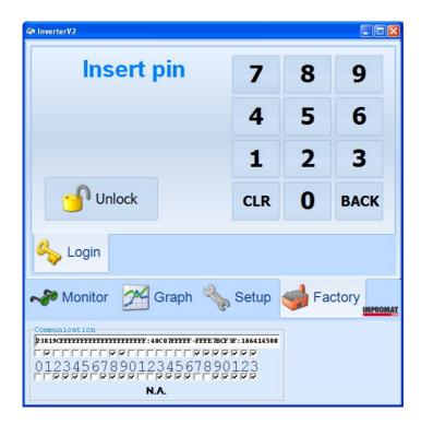
To acces the section "Factory" enter the factory code 1937 and press "Unlock".
