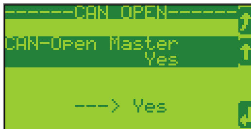
Figure 6-5: Display screen - configure CAN interface
