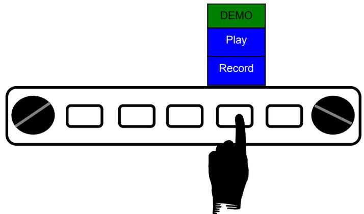
3. To stop the recording locate the **DEMO** button and press **STOP**. Be absolutely certain that a memory stick is in a DU prior to pressing **STOP**. Data is written to internal memory during the flight, and is transferred to the memory stick when **STOP** is pressed.
