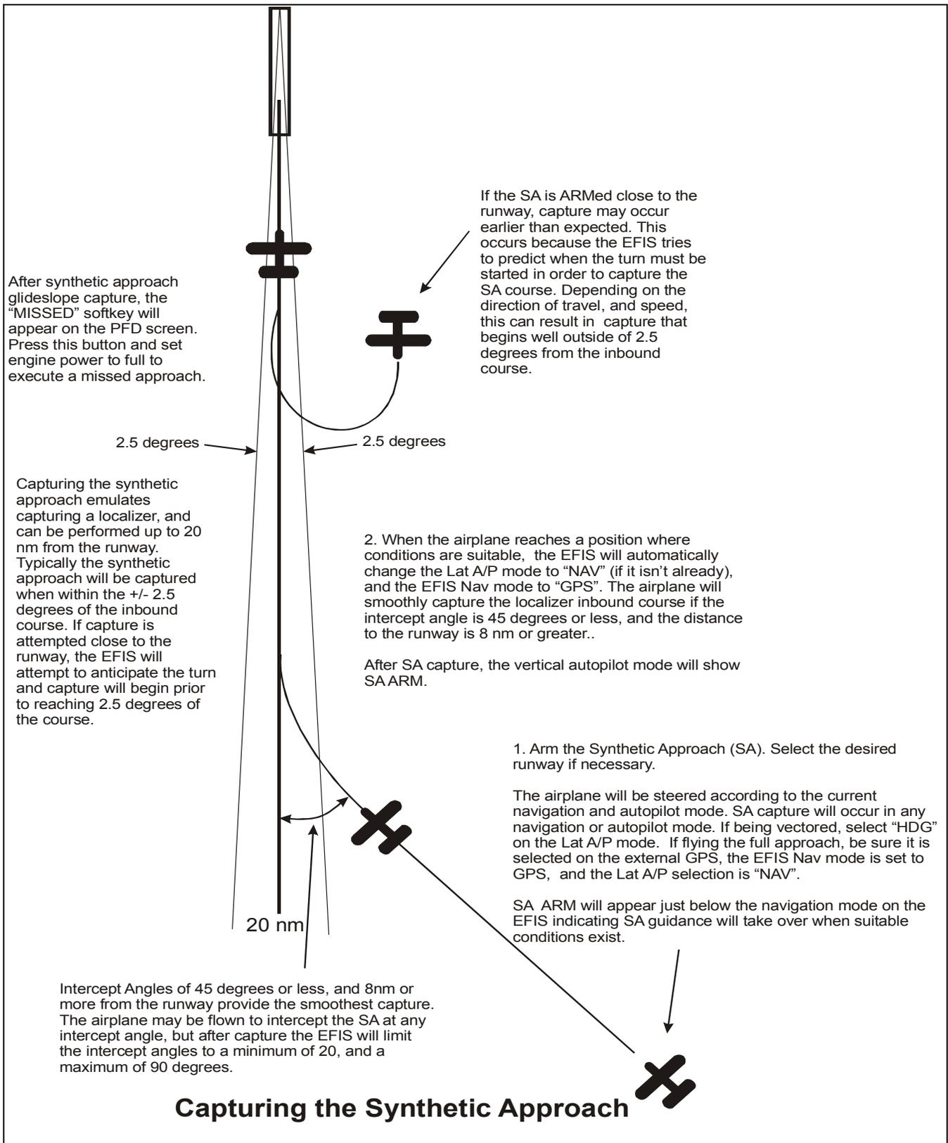
**Fig. 5-1 Synthetic Approach Capture**
