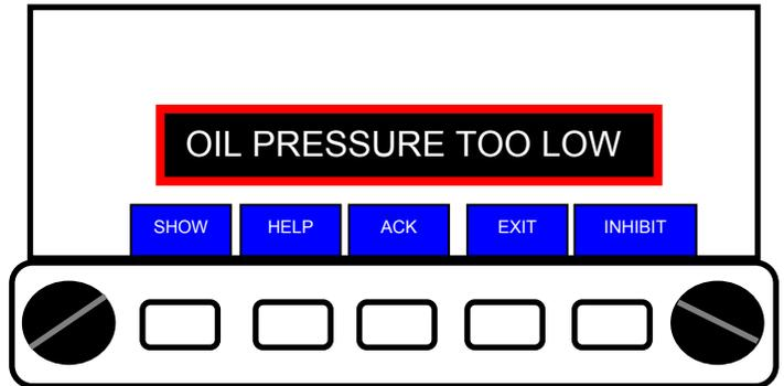
In the example the oil pressure is out of limit, too low. The EFIS will provide five options to choose from.
