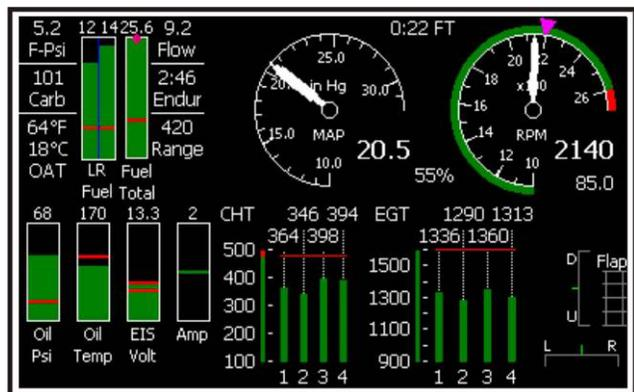
Fig. 4-1 Engine Monitor
