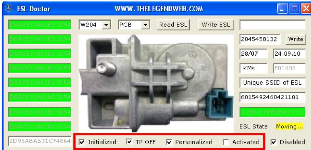
As already noted, when operated in “PCB”-mode for 204-family ESL, it is not possible to issue final “Lock”-command to MCU and it remains non-”Activated”, which leaves the option to program it further when soldered back to original PCB. While ESL is only “Personalized” it is in kind of Test-mode and re-writing with same/another data is possible.
