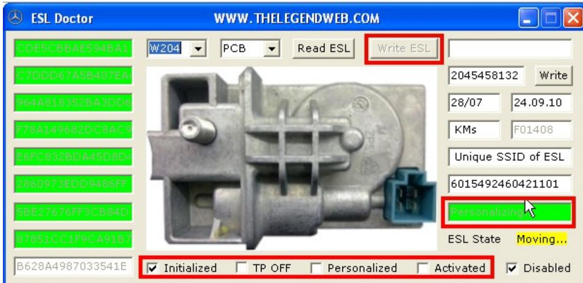
When it is ready software will inform You and will put the ESL in “Locked” position if 204-family ESL is operated in “K-line” mode. If it is in “PCB” mode this command is not issued to MCU and it remains non-“Activated”. The only way to complete adaptation process of that 204-family ESL is to perform it via “K-line”, not while NEC MCU is being placed on adapter board.
