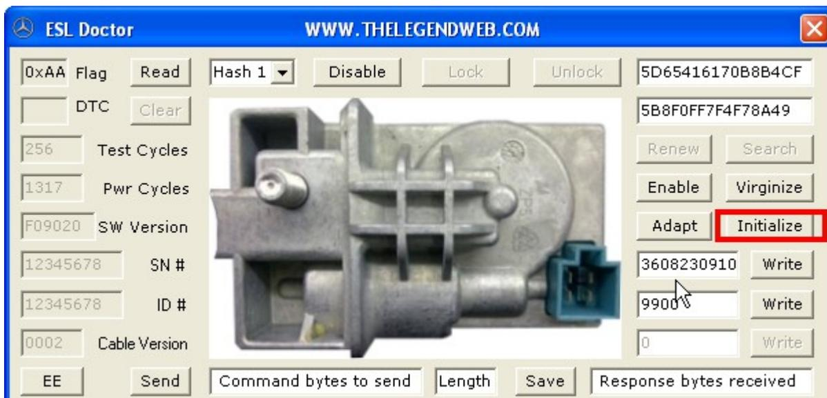
Click “Initialize” button and process starts. Caption is changed to “Stop” making possible to interrupt process at nay desired moment and also progress is indicated:
