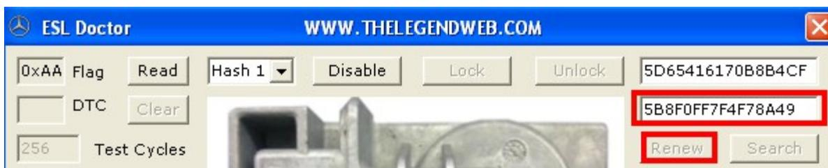
Note that “Renew” button for resetting ESL with Dealer Password is enabled only when ESL allows such action. In example for 204-family ESL it is possible only if working by “K-line” and if ESL has “Activated” and not “Disabled” status!
