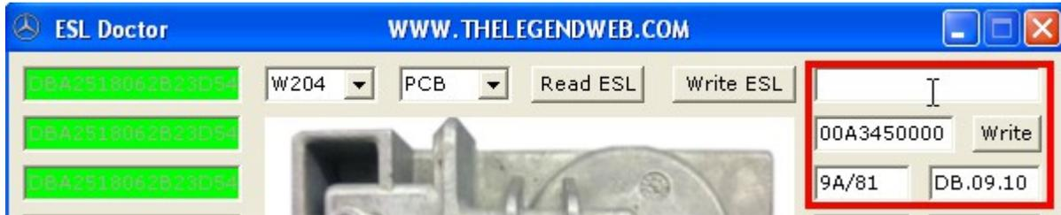
Here, VIN is missing and Part Number and release/software dates values are random. You could enter any desired values, but is advisable to stick to MB-common values, so DAS diagnostics software do not get confused if read this identification information from ESL. Here is an example:
