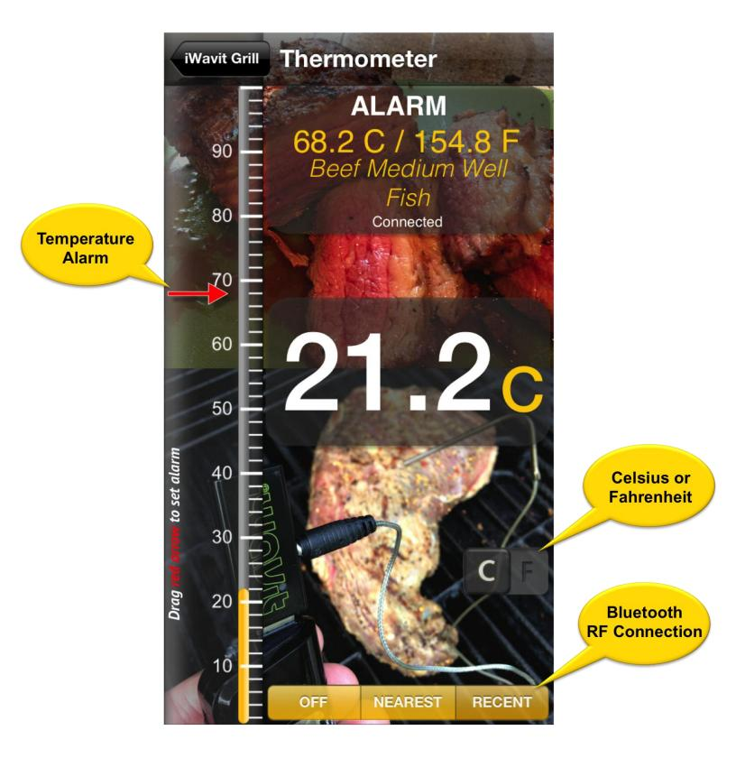
You should now see a screen with the temperature in the middle, presumably close to room temperature. If the reading is not room temperature, make sure that the iWavit temperature plug is plugged in all the way until you hear a "snap".
