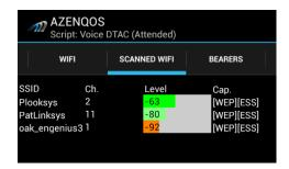
The WIFI panel displays the information of Wi-Fi access points that Android can detect
