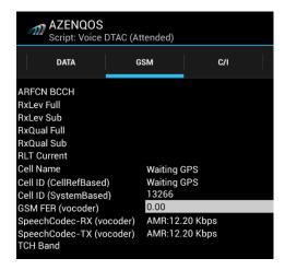
The GSM panel displays the relevant 2G radio parameter and Speech Codec during voice call test
