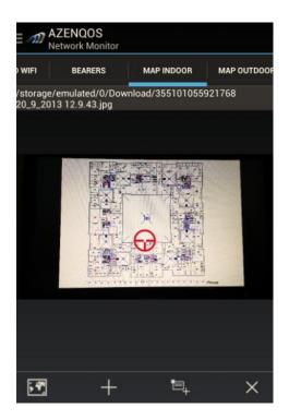
User can pinch to zoom the image for more accurate marking, mark points by moving the target reticle to the desired point and click to add points with tag click.
