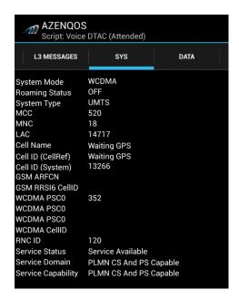
The sys panel displays relevant information about the system the phone is currently latched on to. The Cell ID (System) field will display the Cell ID retrieved from the Android API and may not be accurate, the Cell ID (CellRef) uses the cell reference file in the phone and needs valid GPS location fix to display
