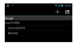
The loop is now setup correctly and starting it will make the phone execute Voice Dial followed by wait for 10,000 times or until the user ends the test
