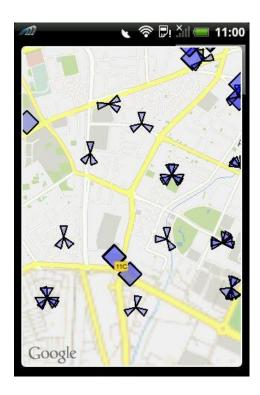
GSM Cell will be displayed in Green/WCDMA cell will be displayed in Blue, Outdoor cells will be displayed in Triangles while Indoors cell will be displayed in squares
