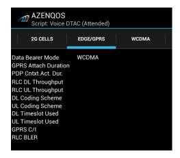
The EDGE/GPRS panel displays the 2G data related radio parameter when Android uses data or conduct data tests
