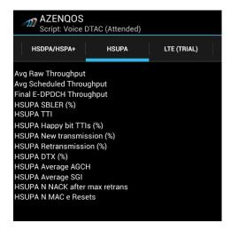
The HSUPA panel displays the 3G data related radio parameter when Android uses data or conduct data tests
