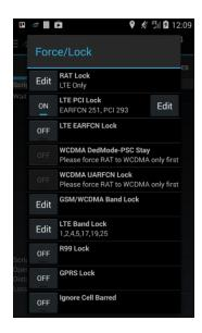
**LTE PCI Lock:** This is LTE 'cell locking'. For testing purposes, engineers can force the phone to use only the specified LTE cell via this feature. Suitable for testing a specifiec LTE Cell in areas where reselections/handovers happen too often or testing the maximum coverage of the cell for cross sector issues.
