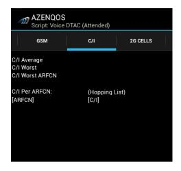
The C/I panel displays the C/I statistics while the phone is in GSM mode
