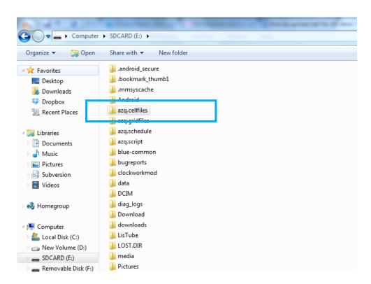
Move your AZQ Cell file into the folder AZQ.cellfiles in the SD card (if it's not found, disconnect the USB cable and enter AZQ again)
