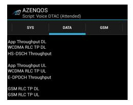
The data panel displays data-related parameters; it will be displayed only when Android uses data connection
