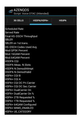
The HSDPA/HSPA+ panel displays the 3G data related radio parameter when Android uses data or conduct data tests
