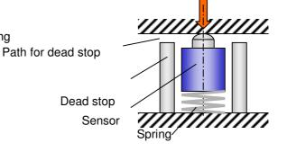
The path for dead stop is determined by the spring. Disadvantage: large measuring path and the sensor must be lead axially.
