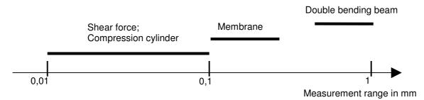
Typical values of the measuring path at force sensors.
